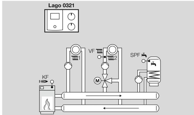
Connect heat source sensor (KF/KFS), flow sensor (VF/VFAS) and storage sensor (SPF/SPFS),
