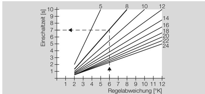
In the case of a controller deviation of 6 K the mixer is actuated for 7s and remains switched off for 3s.
