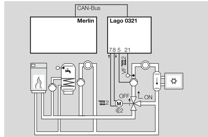
The mixer in the heating circuit functions as a valve. The mixer opens (ON). The heating circuit pump is switched on. P74 = 10.0 – 25.0 °C: The mixer controls to the set flow temperature P74 of the heating circuit, see page 38 (Example: Cooling Operation).
