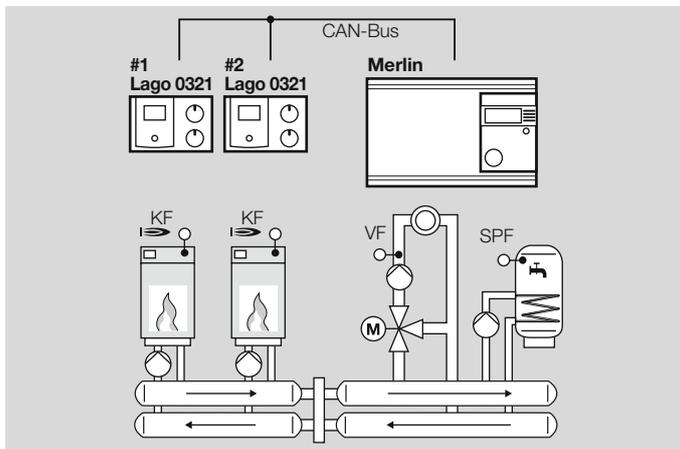
This application is automatically activated as soon as you connect a heat source sensor (KF/KFS) and set parameter 38 = 1–8 (heating module address).
