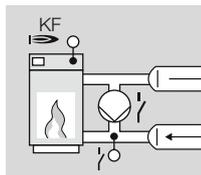
Set P81 and P82 according to boiler manufacturer's specifications
