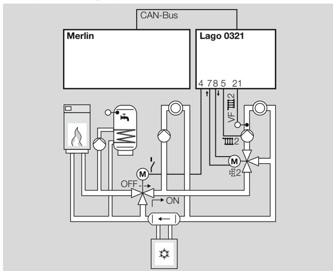
The central controller activates the “Cooling” operating mode via the CAN bus and controls the heat source, the refrigerating machine, the
