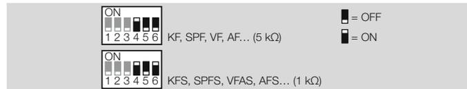
If a remote control is connected, set DIP switch 5:
