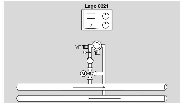
This application is automatically activated if only one flow sensor (VF/VFAS) is connected.
