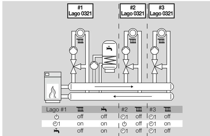
Lago#1 controls the first heating circuit and hot water. Lago #2 controls the second heating circuit and Lago #3 the third. If mode  $\odot$  was selected for Lago #1, the entire system will be switched off, regardless of the settings for the other controllers.
