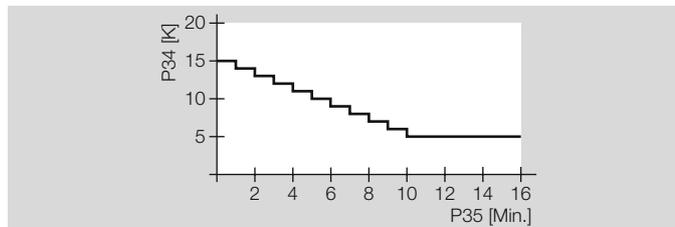
The initial switching hysteresis is reduced from 15 K to 5 K after 10 minutes.
