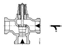
Spindle sealing gland with double O-ring and dirt protection strip.
