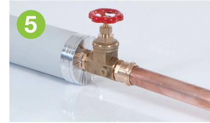
Finishing off the end of the pipe shell with an end capping ensures a tidy appearance. The end cappings are attached to the pipe shell using winding wire or adhesive tape.
