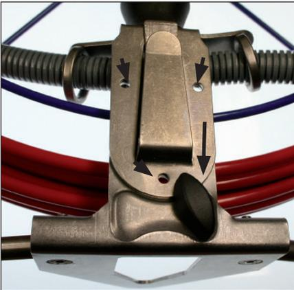
Fix the Viper Stand by turning the black screw to an upright position.
