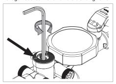
For soft water, turn in the "Soft" direction, for harder water turn to "Hard".
