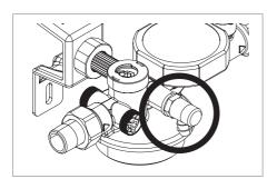
Screw the cartridge under the connection center (2).
