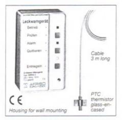
The PTC thermistor oil or water alarm unit sets off visual and audible warning signals in the event of accumulations of liquids which can be caused by tank leaks, backpressure, flooding, etc. The unit consists of an indicator with a built-in operation indicator lamp, an alarm indicator lamp, a buzzer with mute option as well as a flexible PTC thermistor probe. The PTC thermistor probe is mounted at the lowest point of the collecting basin or area to be monitored. The alarm is triggered if the
