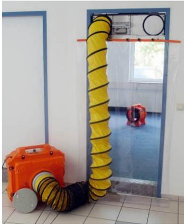
There are now different possibilities of using the Dust Protection System DCS. Depending on the use (see Section 5), filter ventilators can be installed and connected in the white or black area. The DCS is now ready to operate.
